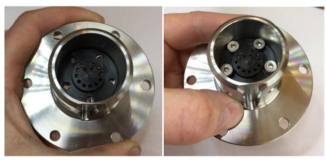
Place the connector into the QR as shown. The two inside pin holes should be opposite the grove on the outside of the QR. Take time to align it properly as an incorrect position will damage your wheel QR when you try and connect it. Now slide the four M4 bolts into place. You only really need two bolts as it's just to hold the connector in place.
