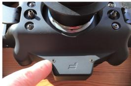
3. Disconnect the shifter cables on both sides.
