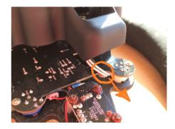
15. The QR will just bolt to the back of the conversion kit. There are 6 threaded holes for a 70mm PCD QR or 3 threaded holes for a 50.8mm PCD one.
