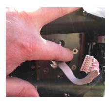
8. Fit the supplied cable to the back of the conversion kit if not already fitted V3.2 needs the cable fitting the correct way around make sure the blue mark on the cable plug lines up with the mark on the kit plug. Version 3.4 can be fitted either way round.
