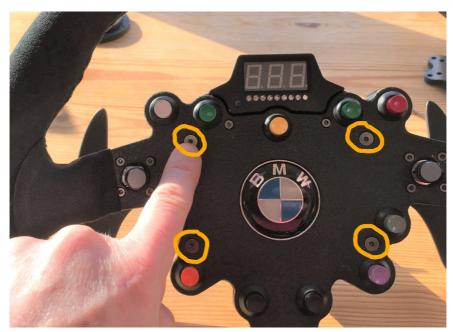
Next on the back of the wheel remove the 2 bolts shown.
