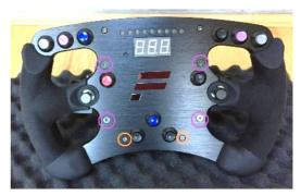
It is advisable to remove the shifter plugs at this stage to make it easier when removing the back of the wheel. Just gently ease both the left and right plugs out.
