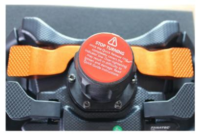
Remove the 6 bolts holding the QR onto the wheel using a 4mm hex key. Then pull the QR off.
