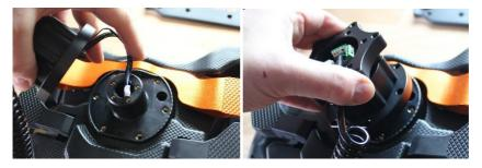
Then put the kit against the wheel and fix with 4 of the bolts removed from the old QR. Remember the wheel is plastic, so do not tighten the bolts too firmly.
