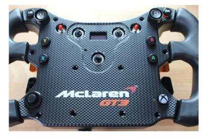
Start by putting the 3 nuts back on the rotary switches. Just hand tight.
