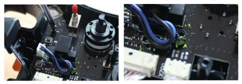
You may find there is green sealent on 2 of the screws. You need to dig this out of the cross head screw to get the driver in. Put all 7 screws aside.
