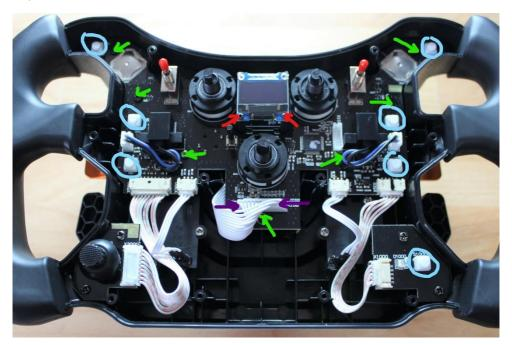
Start by removing all the white button caps so they don't fall off and get lost (shown in light blue) Next, remove the display by undoing the 2 screws marked in red. The display will just lift off.
