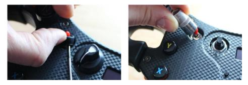
Gently ease the rubber cover off. A small screwdriver helps get it started, then just use your fingers to pull it off. Then undo to nut using an 8mm socket. They are only hand tight. You can leave the nut and washers in situe or remove them.
