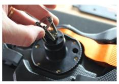
Before you can remove the pin plug you need to bend back the wheel PCB and push the white cable through the wheel.
