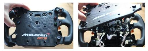
Just pull the cover up. If you left the washers on, be careful to keep it flat. Put the cover asside together with any buttons that may have fallen out.
