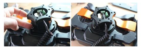
Turn the wheel back over and feed the cable as shown and press it into the PCB socket.
