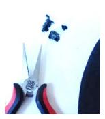
works well. Ensure you do not pull up otherwise the plug and socket will come away from the PCB and may cause damage to the PCB. Alternatively, you can warm the glue with a hair dryer, but this does tend to get messy.
