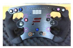
It is advisable to remove the shifter plugs at this stage to make it easier when removing the back of the wheel. Just gently ease both the left and right plugs out.
